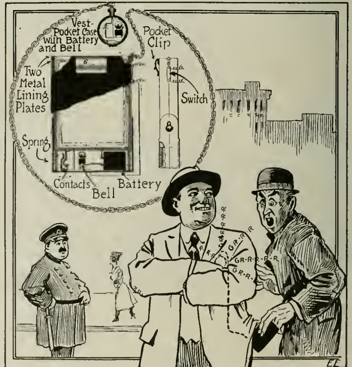
Pickpockets Had Better Beware, for Their Intended Victim May Have His Wallet Protected By This Newly Patented Electric Alarm. When the Purse Or Wallet is Touched the Bell Rings.
