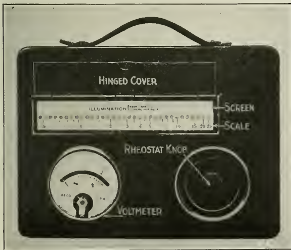
An Extremely Simple Foot-Candle Meter Recently Brought Out.
